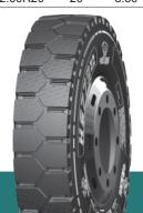
Special designed mine pattern tyre for harsh road ,with wide tyre crown and deep tread, which could provide higher mileage. The large lateral pattern block can produce the driving forces, maintaining excellent grip performance both in the dry and wet pavem.
